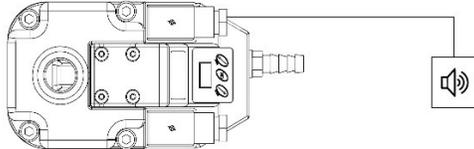
1. Unscrew the connector screw and remove the cap from the alarm connector to connect the alarm cables to the connector as shown below. Caution is required as you may be working with hazardous voltages!
