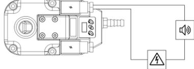
2. Connect the cable to your alarm device, any device of your choice can be applied i.e. a (flashing) light or alarm panel.
