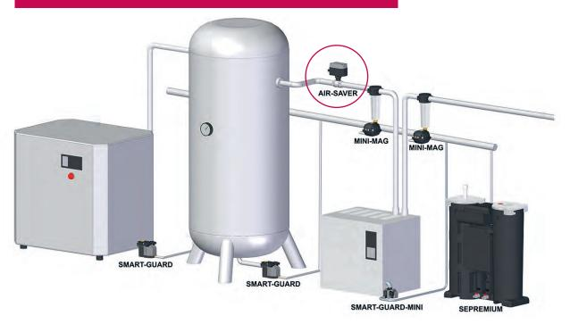
The AIR-SAVER typically gets installed after the receiver (air tank). Once closed, it retains the compressed air built up in the receiver and ensures that the compressor does not run unnecessarily during moment when it is not required.
