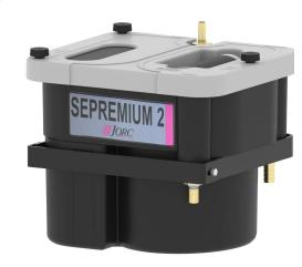
As soon as the condensate enters the SEPREMIUM 2 Serviceable, it is filtered through the various filter elements. The oil absorbing elements combine different types of adsorption technologies, assuring a result of less than 5 ppm residual oil content at the exit can be achieved.
