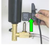
7. Replace the valve parts with the parts supplied in the service kit.
