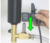
6. Unscrew the valve shaft using a 23 mm wrench.
