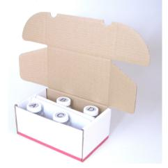
4. Shake the condensate (0,5L) and then fill all four test bottles with condensate (approx. 100ml each).
