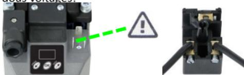
3. Connect your alarm device to a power supply. The alarm switch type is a 'contact output switch'. An external power supply is required as the alarm connection point on the drain works like a relay switch only.
