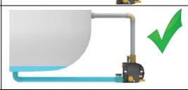
Do not narrow the feed pipe when installing additional adapters or piping, these may cause air locks.
