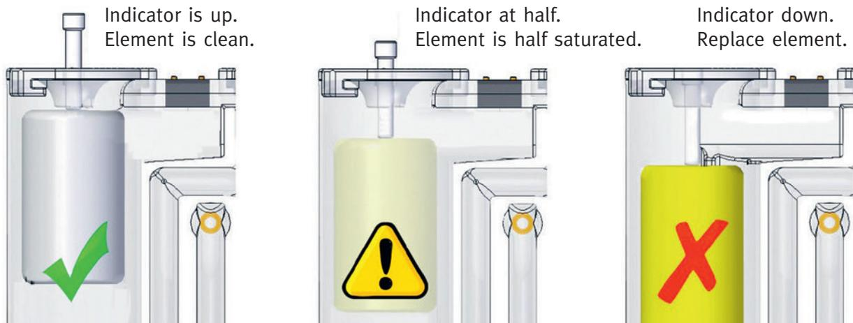
One unique feature of the SEP premium separators is the element life indicator (white). This indicator gives instant visual confirmation of the condition of the elements in the separator and when they need to be replaced.
