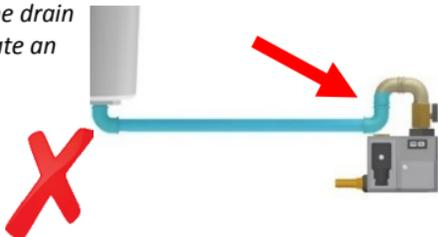
The 1/2" drain pipe must be horizontal or ideally at a downwards slope ( $>1^\circ$ ).
