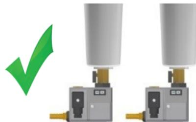
Avoid water pockets when installing the drain pipe, this will create an air lock.
