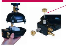
The POD-TD design allows you to service the valve by unthreading one brass fitting. You have direct access to the valve plunger and orifice.
