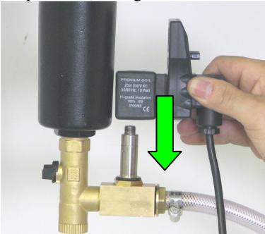
6. Unscrew the valve shaft using a 23 mm wrench.
