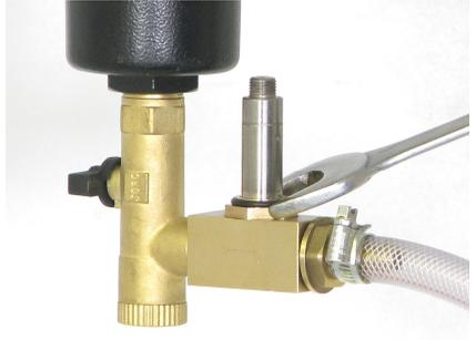
*Do not use the valve shaft as lever!*
