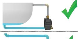
Do not narrow the feed pipe when installing additional adapters or piping, these may cause air locks.
