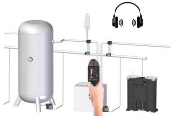
Visual and audible leak indication
